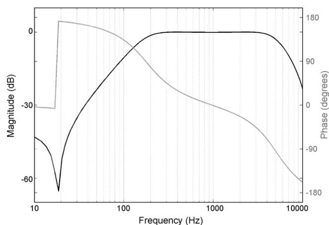
Fig. 1. Magnitude and phase response of a fourth order band-pass elliptic filter between 300 and 3000 Hz.
