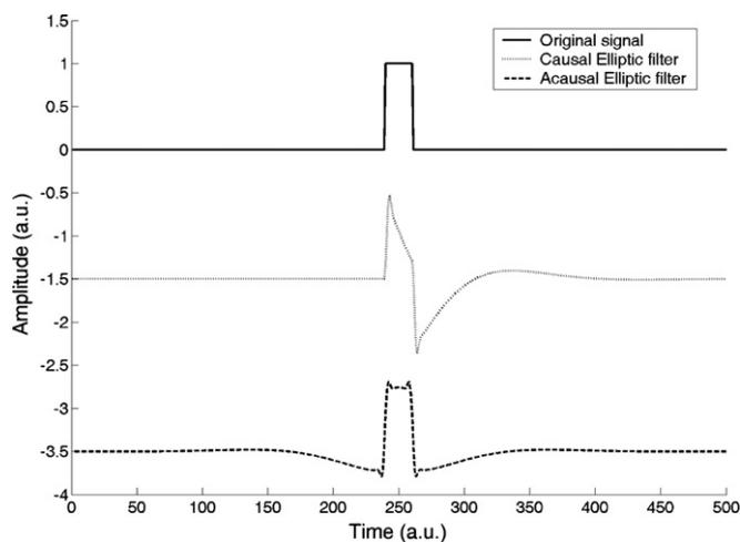
Fig. 2. Example of filtering distortions introduced by causal filters. The causal elliptic filter introduces asymmetric distortions and the filtered signal barely resembles the original pulse. Distortions are smaller with the noncausal implementation of the same elliptic filter.
