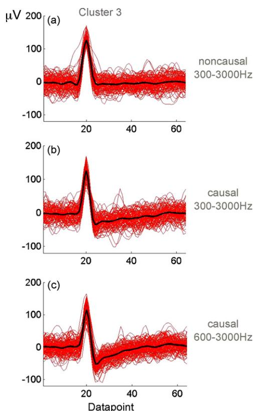
**Fig. 5.** A pulse artifact detected with the same filter settings of the previous figure. Note that the causal filter distorts the shape of the artifact and makes it look similar to a real spike.
