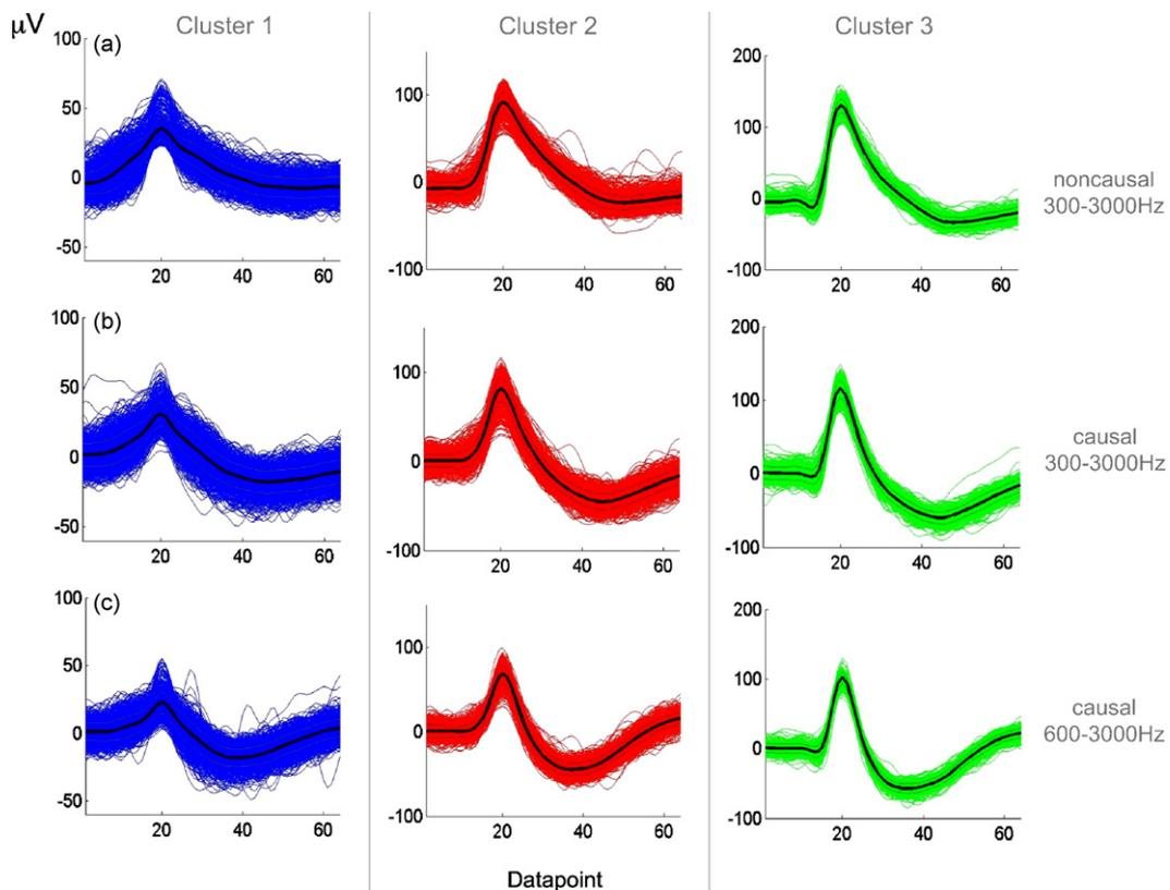
**Fig. 4.** The 3 clusters of spike shapes obtained from the previous figure, detected using different filters: (a) noncausal filter between 300 and 3000 Hz, (b) causal filter between 300 and 3000 Hz and (c) causal filter between 600 and 3000 Hz. Note the distortions of the spike shapes introduced by the causal filters.
