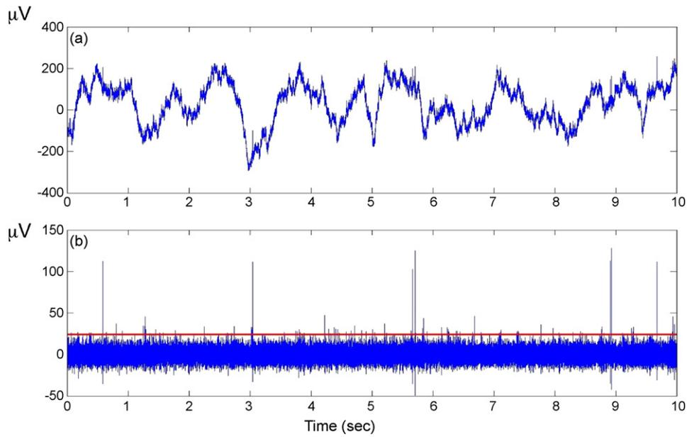
**Fig. 3.** (a) Ten seconds of a continuous recording from a microwire in the medial temporal lobe of a human subject. The raw data is dominated by low frequency activity and it is very difficult to visualize the spikes. (b) The same recording after band pass filtering. Note that spikes can now be easily detected with an amplitude threshold (horizontal line).
