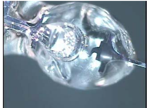
Figure 5. Electrolysis inside the parylene balloon of the actuator.
